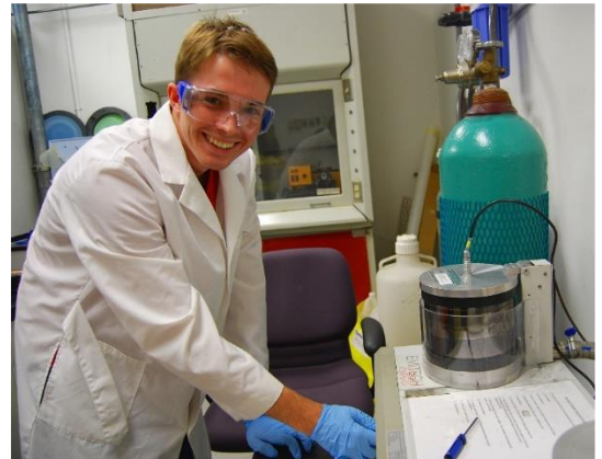
Jayk sputter coats samples in preparation for scanning electron microscope imaging.
