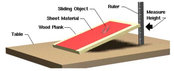
This test will help determine at what angle a sample piece of material starts to slide. The steeper the hill, the more friction there is between the test piece and the material covering the slope. The more friction, the worse those materials are for bearings. The lower the friction, the sooner the object will start to slide and the smaller the angle will be.
